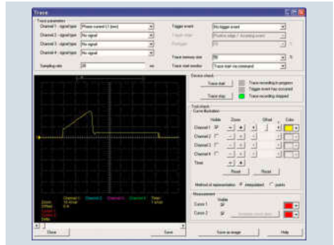
Graphic presentation of measured values with the trace function (oscilloscope function) of Soft Starter ES 2007 Standard and Premium
