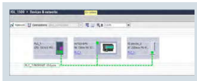
Configuration of a PROFINET network with lower-level IO-Link masters
