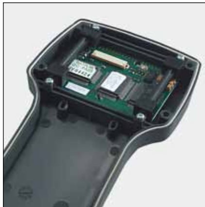
Display fixing set for variable display mounting
