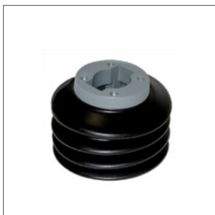
Inclining adapter Cast aluminium part with bellow and seal, inclination can be adjusted to any angle between 0° and 45°. Screw-mounted between enclosure and coupling.
