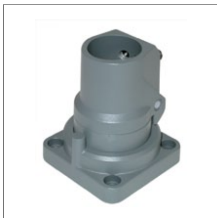
Foot stand, turnable Cast aluminium with steel inner tube and flange mounting. Swivelling range 250° (cannot be limited or stopped)
