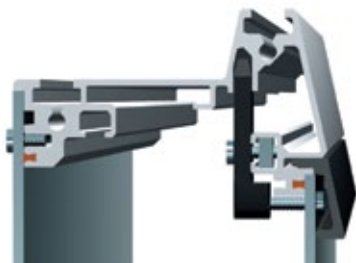
Front panel installation screwed from front
