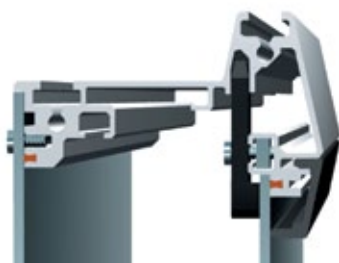
Front panel installation from rear
