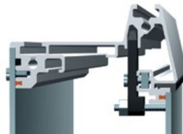
Front panel installation with stud bolts
