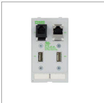
RJ45; RJ12; USB; USB (type A) 1 × RJ45, 8-pole. Metal, CAT5e (socket/socket); 1 × RJ12, 6-pole. Plastic; 2 × USB (socket/socket) Type A
