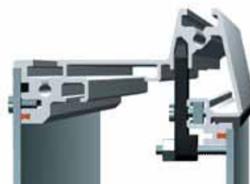
Front panel installation with stud bolts
