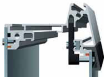
Front panel installation screwed from front
