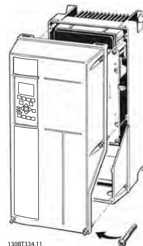
Illustration 3.9 Control Wiring Access for IP55 / Nema 12 and IP66 / Nema 4/4X Indoor
