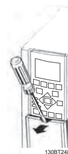
Illustration 2.8 Control Wiring Access for IP20 / Open chassis enclosures
