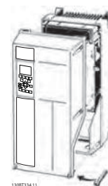
Illustration 2.9 Control Wiring Access for IP55 / Nema 12 and IP66 / Nema 4/4X Indoor
