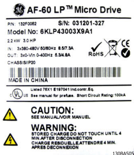
Figure 2.1 This Example Shows the Nameplate Sticker
