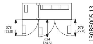
Illustration 4.11 Space in front of IP21/Nema 1 and IP54/Nema drive types for unit size 62.
