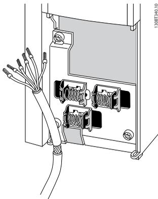
Connect the wires as described in the Operating Instruction for the frequency converter. Remember to connect the shields in a proper way to ensure optimum electrical immunity.
