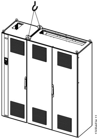
**Illustration 4.4 Recommended Lifting Method, Unit Size 62**
