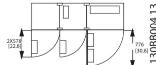
Illustration 4.10 Space in front of IP21/Nema 1 and IP54/Nema drive types for unit size 63.
