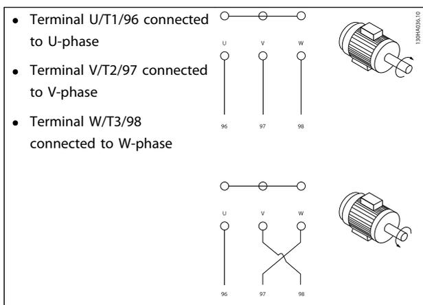
The direction of rotation can be changed by switching two phases in the motor cable or by changing the setting of *H-08 Reverse Lock* and reversing.
