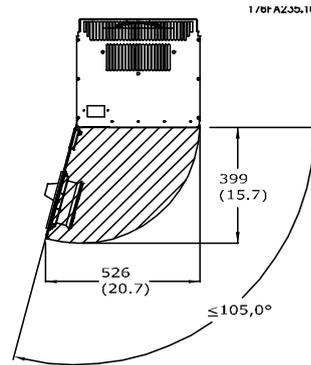
Illustration 4.7 Space in front of IP21/Nema 1 and IP54/Nema 12 drive in unit sizes 41 and 42.
