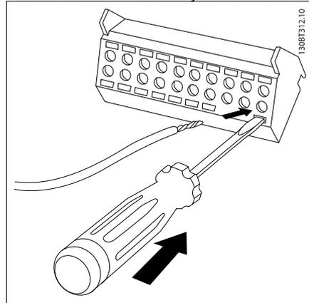
4. Remove the screwdriver. The cable is now mounted in the terminal.
