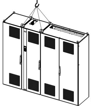
**Illustration 4.6 Recommended Lifting Method, Unit Size 64**
