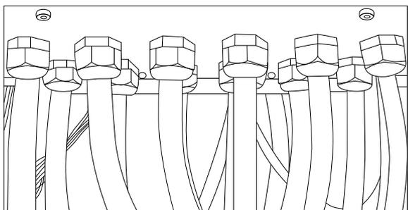
Illustration 4.31 Example of Proper Installation of Gland Plate.
