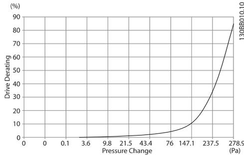
**Illustration 4.27 Unit Size 5X Derating vs. Pressure Change (Small Fan), 350 HP @ 460V and 500-550 HP @ 690 V**
