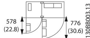
Illustration 4.9 Space in front of IP21/Nema 1 and IP54/Nema drive types for unit size 61.
