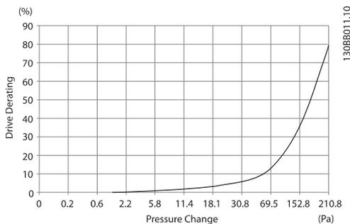
**Illustration 4.28 Unit Size 5X Derating vs. Pressure Change (Large Fan)**
