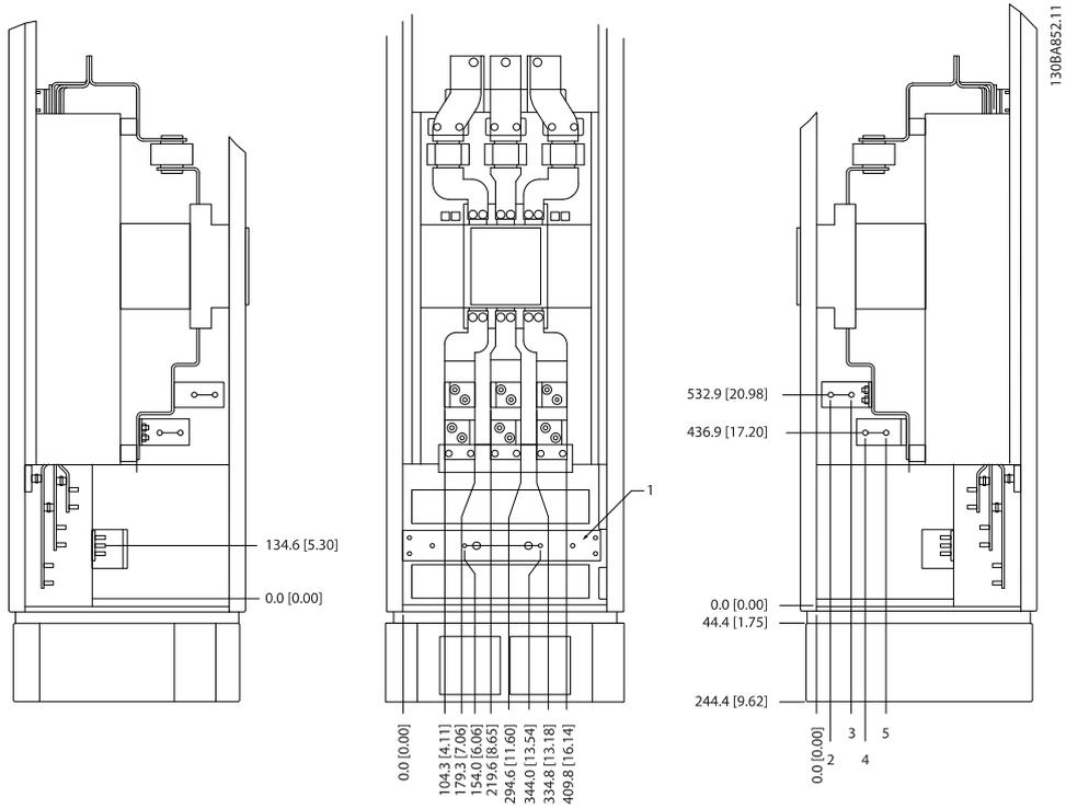
Illustration 4.25 Terminal locations - Options Cabinet with circuit breaker/ molded case switch (Left side, front and right side view). The gland plate is 42 mm below .0 level.
