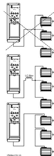
Problems may arise at start and at low RPM values if motor sizes are widely different because small motors' relatively high ohmic resistance in the stator calls for a higher voltage at start and at low RPM values.
