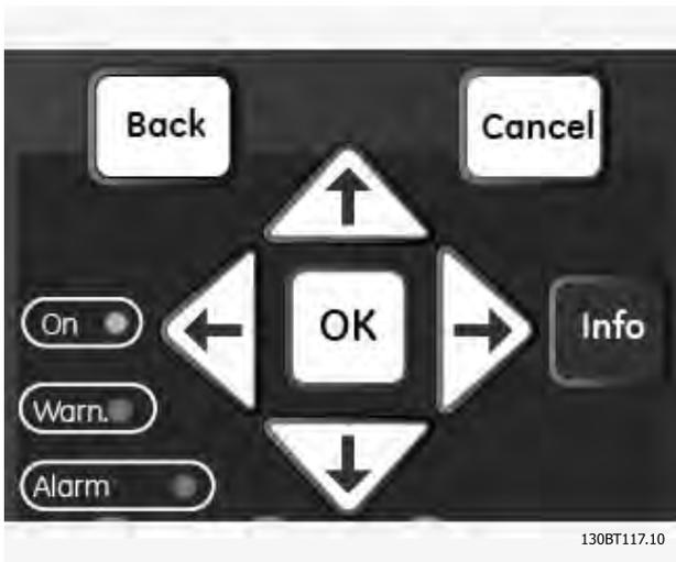
Operation Keys for local control are found at the bottom of the keypad.
