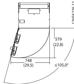
Illustration 4.8 Space in front of IP21/Nema 1 and IP54/Nema drive types for unit size 51.
