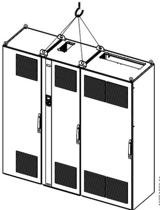
**Illustration 4.5 Recommended Lifting Method, Unit Size 63**
