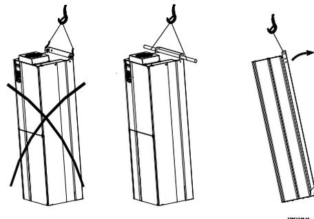
**Illustration 4.30 Lifting method for mounting drive on wall**
