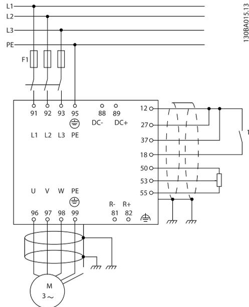
**Illustration 4.1** Diagram showing basic installation including mains, motor, start/stop key, and potentiometer for speed adjustment.
