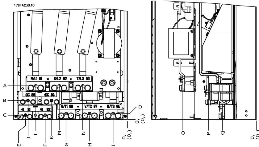
Illustration 4.13 Position of power connections, 43/44 Unit Sizes
