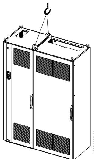
Illustration 4.3 Recommended Lifting Method, Unit Size 61 (460V, 600 to 900 HP, 575/600V, 900 to 1150 HP).
