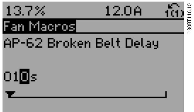
Illustration 6.7 Step 6: Use the up/down navigation keys to change the delay time.
