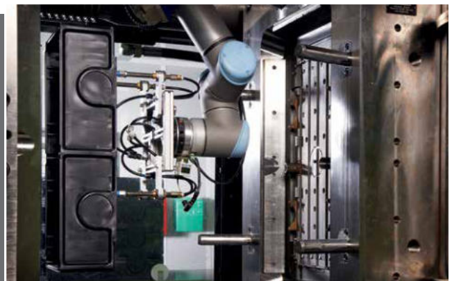
Automatic removal process for our VARIABOX system
